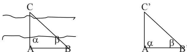
2. The distance of the point A from the point B, if the length AB cannot be measured directly.
