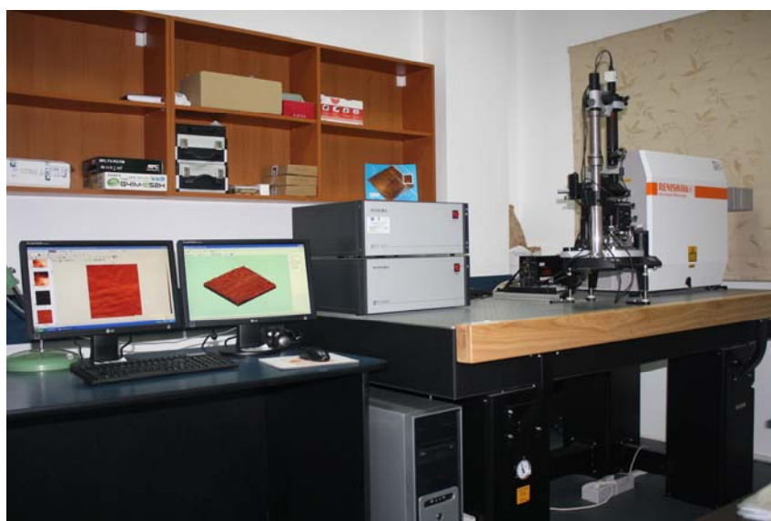
Figure 1. Atomic Force Microscope coupled with confocal Raman spectroscopy used at ICDISTN of “Aurel Vlaicu” University.
