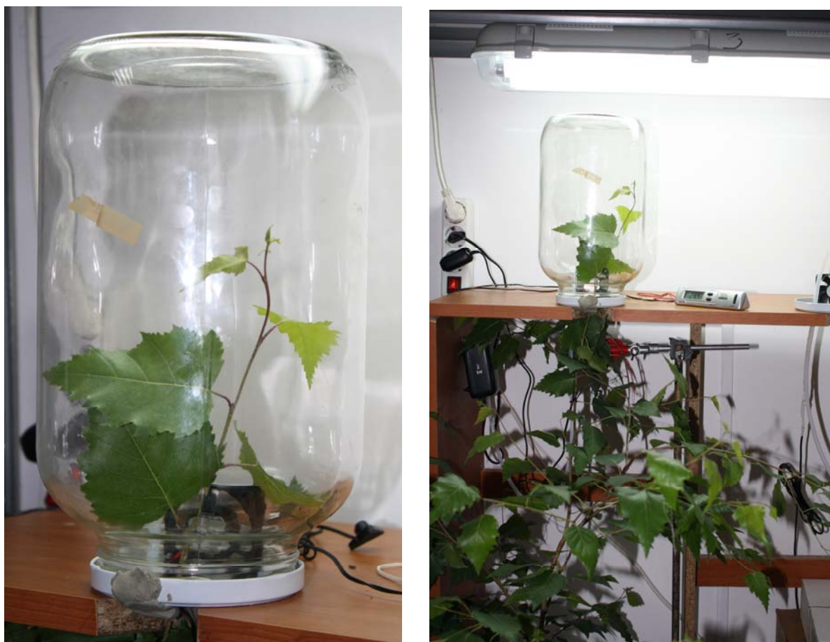
Figure 1. Custom-built system for measuring volatile organic compounds
