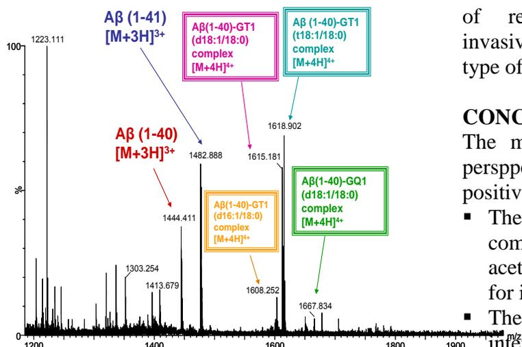
**Figure 4.** NanoMate-QTOF MS in positive ion mode of the reaction products resulted after 30 min incubation in buffer at 37 °C of A $\beta$  protein and human brain GG mixture. Acquisition time: 5 min. nanoESI: 1.4 kV; cone voltage: 50 V; nitrogen at 0.40 psi. Buffer system: 10 mM ammonium acetate/acid acetic pH 6.0.
