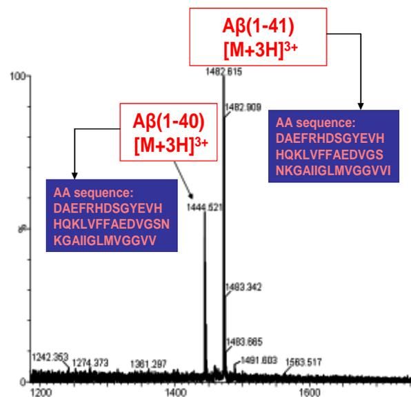
**Figure 3.** NanoMate-QTOF MS in positive ion mode of the A $\beta$  protein in buffer. Concentration: 1 pmol  $\mu\text{L}^{-1}$ ; acquisition time 2 min. nanoESI: 1.2 kV; cone voltage: 50 V; nitrogen at 0.40 psi. Buffer system: 10 mM ammonium acetate/ acetic acid pH 6.0.
