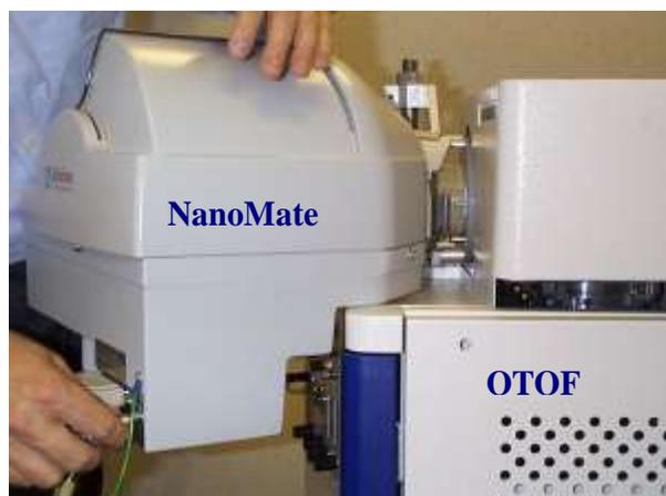
**Figure 1.** Chip-based nanoelectrospray, NanoMate™ robot incorporating the 400-nozzle ESI Chip technology (Advion BioSciences, Ithaca, USA) in laboratory coupled to a QTOF MS (Waters, Manchester, UK). The electrospray process was initiated at 1.3 kV applied on the pipette tip and 0.40 psi nitrogen back pressure
