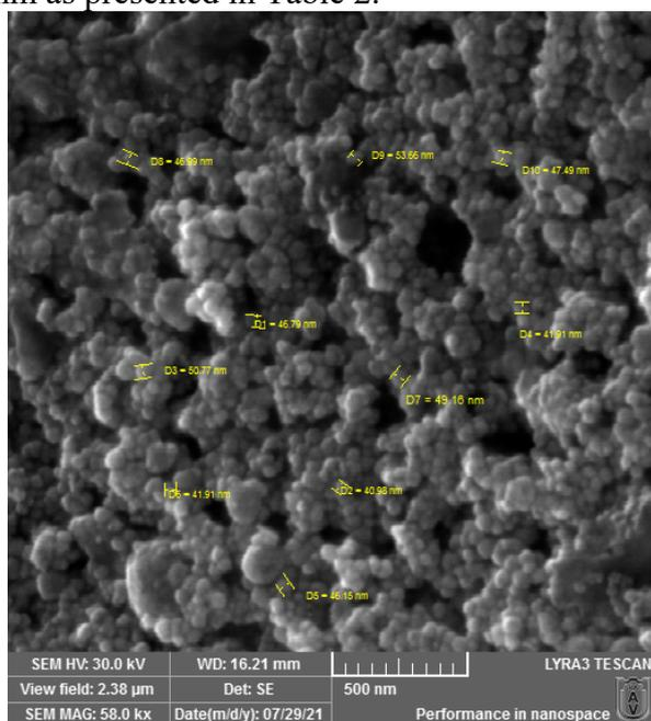
**Figure 4.** SEM micrograph of the hydrolat biosynthesized AgNPs
