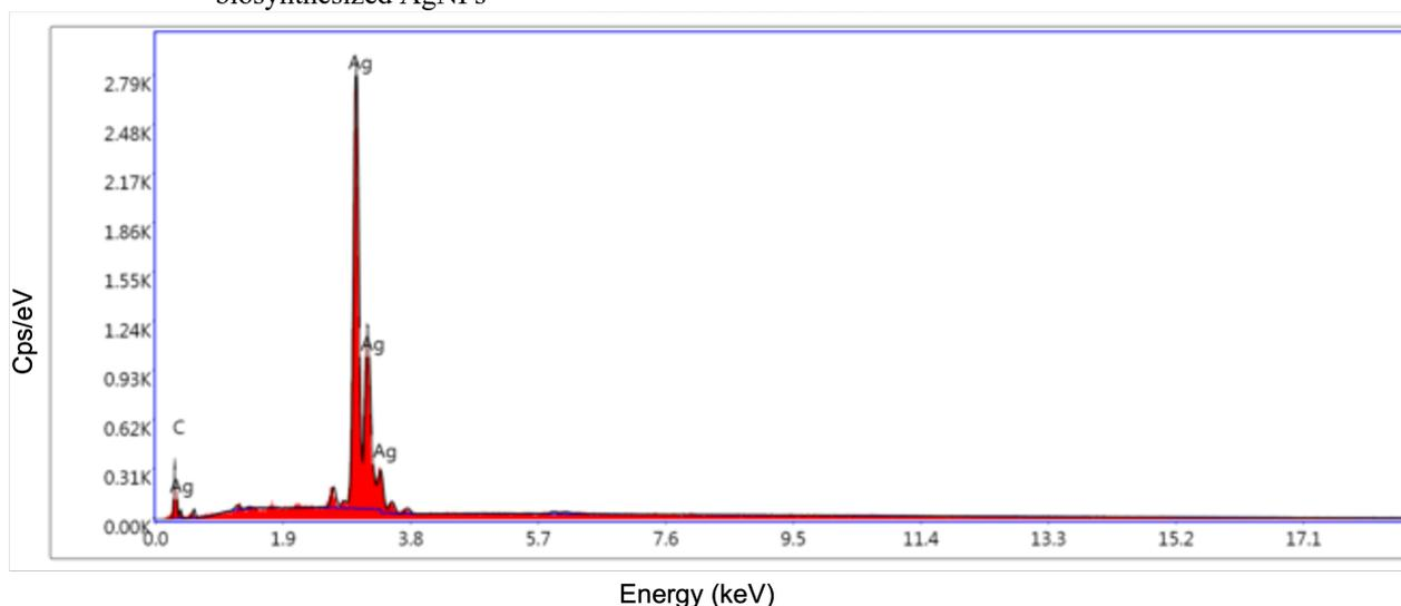
**Figure 5.** EDX spectrum of the hydrolat biosynthesized AgNP
