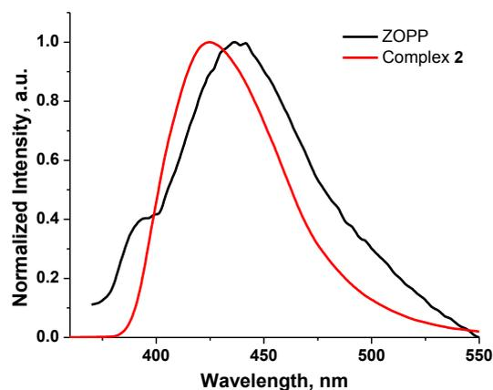
**Figure 3.** Normalized photoluminescence spectra of free ligand and complex 2
