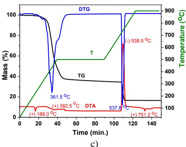
**Figure 4.** Thermal decomposition of: a) the ligand (ZOPP), b) Ni(ZOPP-2H) and c) Zn<sub>2</sub>(ZOPP-2H)(CH<sub>3</sub>COO)<sub>2</sub> in nitrogen/air condition.
