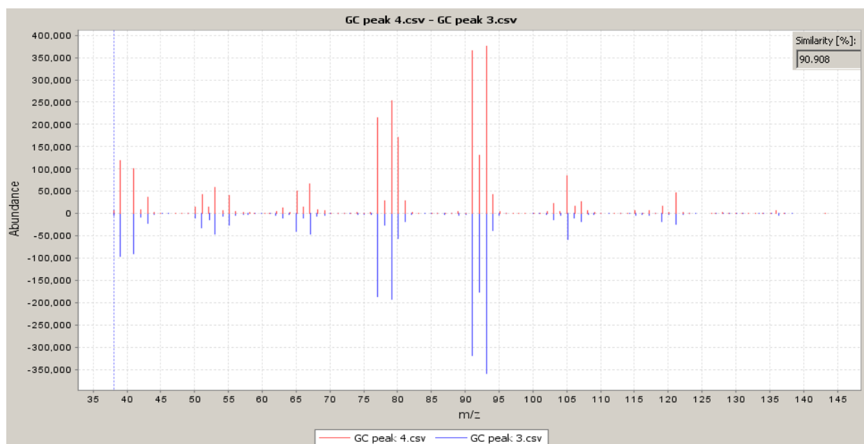
Figure 2. The mirrored mass spectra of GC peak 4 (above) and GC peak 3 (down)
