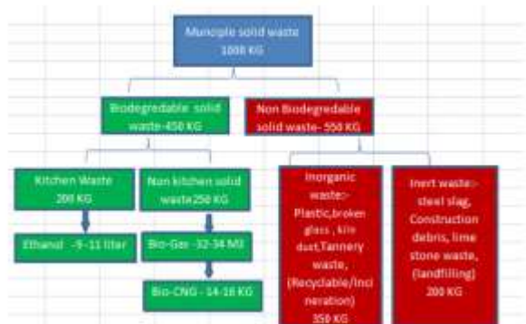
Figure 1. Composition of municipal solid waste that can be treated as a source for production of the necessary energy. From (Soni et al., 2016)
